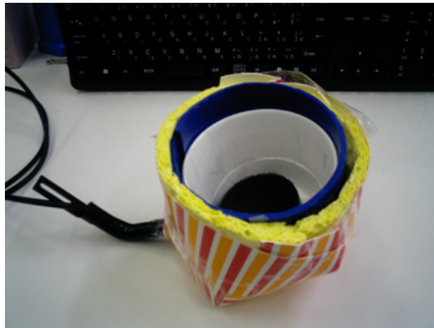
Figure 4.15: Test production of a nonmagnetic microphone cover for noise reduction within the gantry
